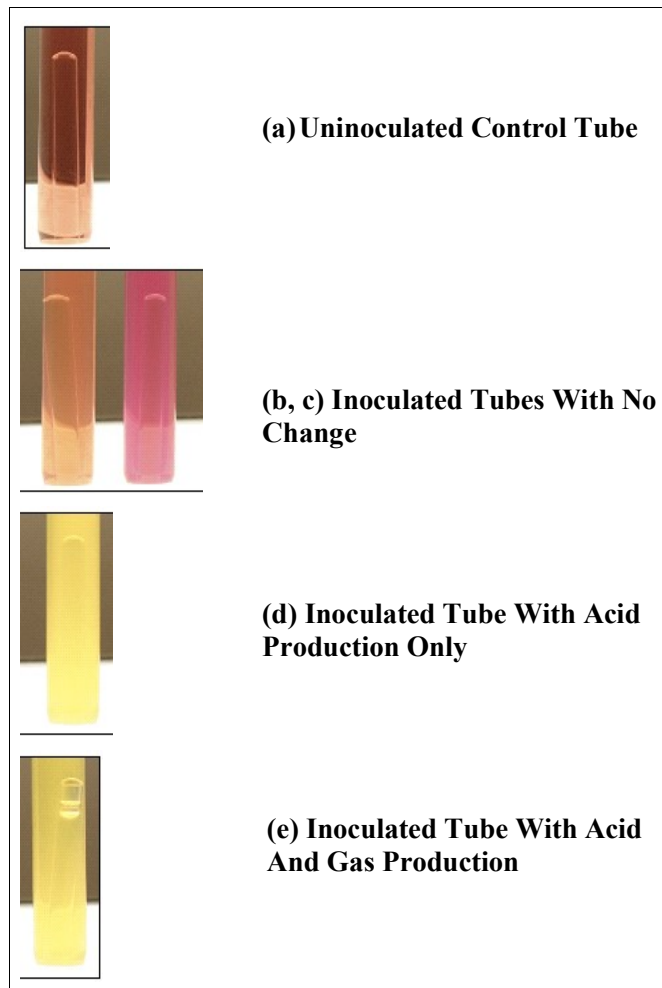
Fig. 2: Possible MPN Presumptive Test Results
